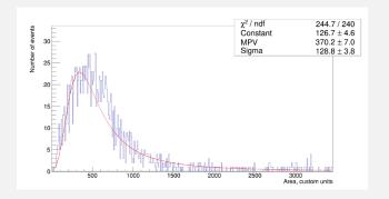
• The signal loss is very dramatic, however, its still possible to do the MIP calibration and the dynamic range is increased.
