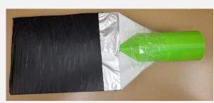
Shown are the completed paddle and the layers exposed. The PMT connector part is 3D-printed. The scintillator is covered by Tyvek for higher light yield. Additionally, aluminum foil, insulation tape, and duct tape were added for both light insulation and structural support.
